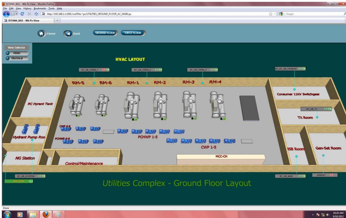
Chiller Room at Utility Block
